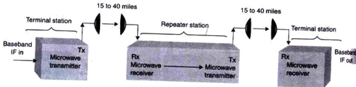
The repeater station receives a signal, amplifies and reshapes it, and then retransmits it to the next repeater or terminal station down line from it. A terminal station is simply a station at the end of a microwave system where information signals originate and terminate.
