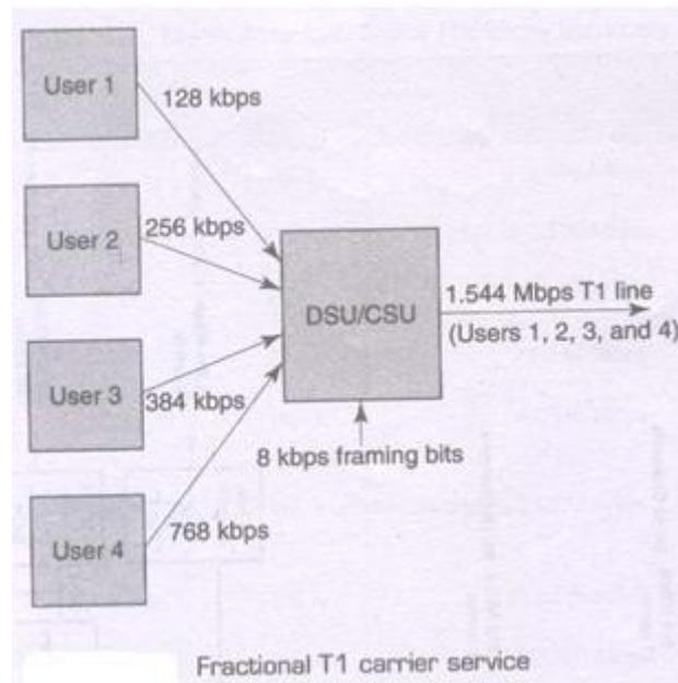
The above figure shows four subscribers combining their transmissions in a special unit called a *data service unit/channel service unit* (DSU/CSU). A DSU/CSU is a digital interface that provides the physical connection to a digital carrier network. User 1 is allocated 128 kbps, user 2 - 256 kbps, user 3 - 384 kbps, and user 4 - 768 kbps for a total of 1.536 kbps (8 kbps is reserved for the framing bit).
