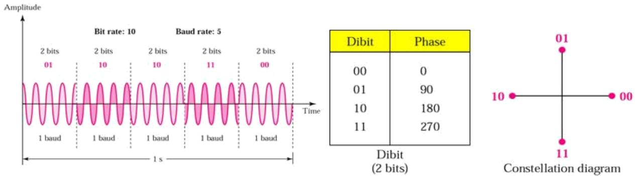
The above figure shows the output phase-versus-time relationship, truth table, and constellation diagram for QPSK. A phase of  $0^\circ$  now represents 00;  $90^\circ$  represents 01;  $180^\circ$  represents 10; and  $270^\circ$  represents 11. Data can be transmitted twice as efficiently using 4-PSK than 2-PSK.
