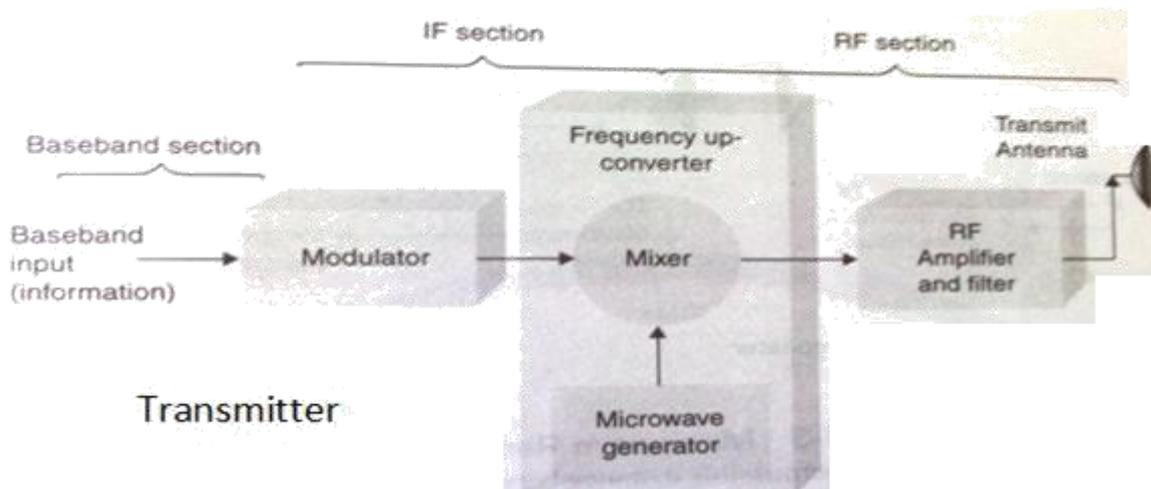
The modulator may perform frequency modulation or some form of digital modulation such as PSK or QAM. The output of modulator is an intermediate frequency (IF) carrier that has been modulated or encoded by the baseband input signal. The baseband signal is simply the
