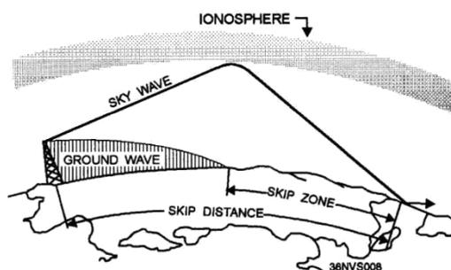
The SKIP ZONE is a zone of silence between the point where the ground wave becomes too weak for reception and the point where the sky wave is first returned to Earth. The size of the skip zone depends on the extent of the ground wave coverage and the skip distance. When the ground wave coverage is great enough or the skip distance is short enough that no zone of silence occurs, there is no skip zone.
