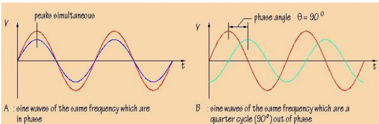
A phase shift of 360 degrees corresponds to a shift of one complete cycle. If two sine waves have the same frequency and occur at the same time, they are said to be **in phase**, or they are said to out of phase. The difference in phase can be measured in degrees, and is called the **phase angle, Ø**
