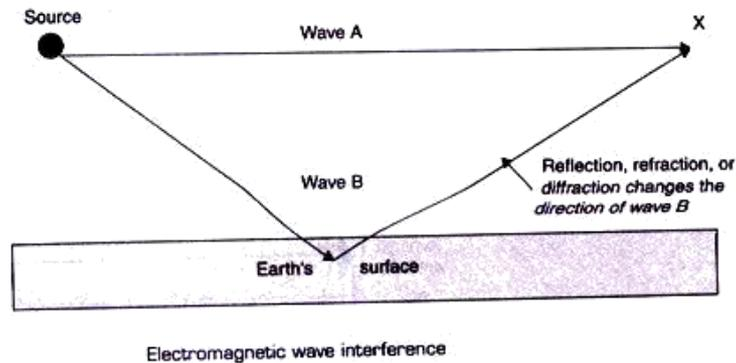
In the above figure, it can be seen that, at point X the two waves occupy the same area in space. However, wave B has travelled a different path than wave A and, therefore, their relative phase angles may be different. If the difference in distance travelled is an odd-integral multiple of one-half wavelength, reinforcement takes place. If the difference is an even-integral multiple of one-half wavelength, total cancellation occurs.
