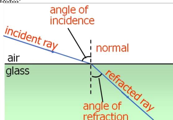
When an electromagnetic wave is reduced as it passes from one medium to another medium of denser material, the light ray changes direction or refracts (bends) toward the normal. When an electromagnetic wave passes from a more dense material into a less dense material, the light ray is refracted away from the normal. The normal is simply an imaginary line drawn perpendicular to the interface of the two materials at the point of incidence
