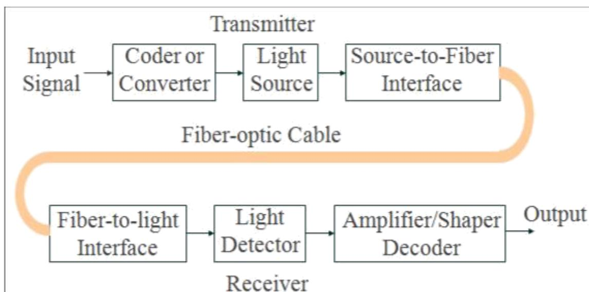
The three primary building blocks are transmitter, receiver and the optical fiber cable. The transmitter is comprised of a voltage-to-current converter, a light source, and source-to-fiber interface. The fiber guide is the transmission medium, which is either an ultrapure
