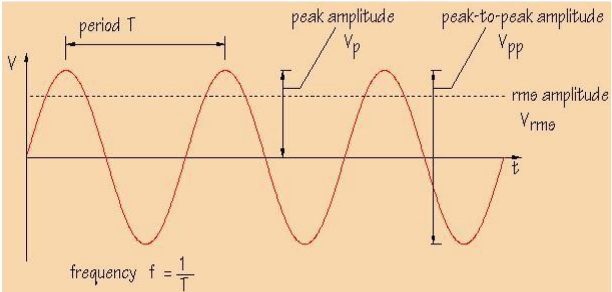
**Frequency (f):** The time of one cycle of a waveform is its period, which is measured in seconds. Frequency is the number of cycles completed per second. The measurement unit for frequency is the **hertz, Hz**. 1 Hz = 1 cycle per second. The frequency of the signal can be calculated from  $T=1/f$
