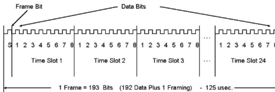
As a result of this extra bit, each frame now contains 193 bits and the line speed for a T1 digital carrier system is 1.544 Mbps. { 193 bits × 8000 frames = 1.544 Mbps }
