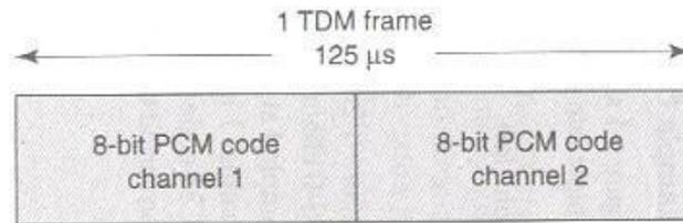
The multiplexer is simply an electronically controlled digital switch with two inputs and one output. One eight-bit PCM code from each channel is called a TDM frame and the time it takes to transmit one TDM frame is called frame time and it is equal to reciprocal of sample rate. The above figure shows the frame allocation for a two channel PCM system. The PCM code for each channel occupies a fixed time slot within the total TDM frame.
