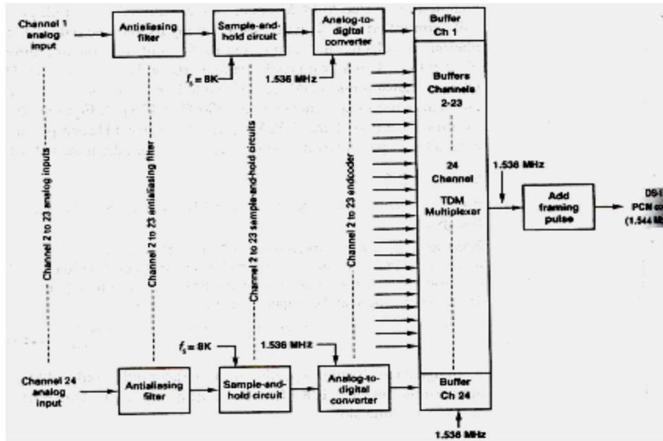
A T1 carrier system time division multiplexes PCM encoded samples from 24 voice band channels for transmission over a single metallic wire pair or a fiber optic cable. The multiplexer has 24 independent inputs and one time-division multiplexed output. The 24 PCM output signals are sequentially selected and connected through the multiplexer to the transmission line. To become a T1 carrier, the system has to be line encoded and placed on special conditioned cables called T1 lines.
