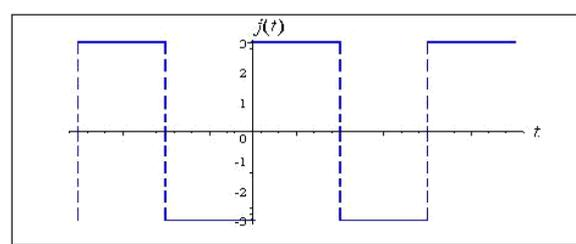
**Odd symmetry:** If a periodic voltage waveform is symmetric about a line midway between the vertical axis and the negative horizontal axis and passing through the coordinate origin, it is said to have to point or skew, symmetry and is called an odd function. For all odd functions, the  $\alpha$  coefficients are zero. Odd function satisfies  $f(t) = -f(-t)$
