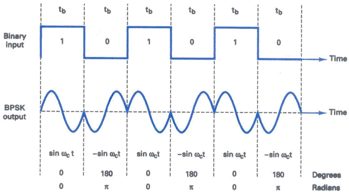
**FIGURE 9-15** Output phase-versus-time relationship for a BPSK modulator
