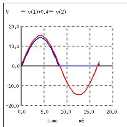
**Half-wave symmetry:** If a periodic voltage waveform is such that the waveform for the first half cycle repeats itself except with the opposite sign for the second half cycle, it is called to have half-wave symmetry. Half-wave symmetry implies that the second half of the wave is exactly opposite to the first half. A function with half-wave symmetry does not have to be even or
